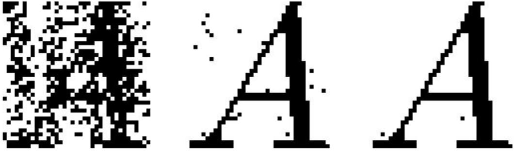
Figure 4.9: Bitonal image reconstruction results using BP(left), SAV(middle), and proposed BRSN(right)
